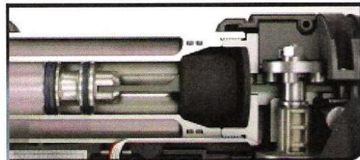
3 Motor turns lifter which resets piston
