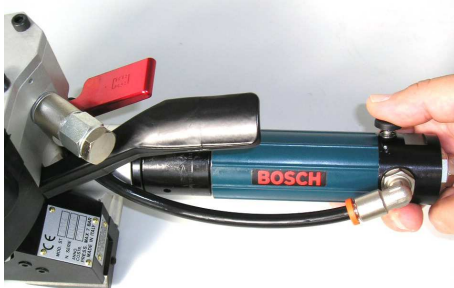
PHASE 1 : STRAP TENSIONING
